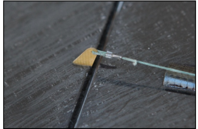
Figure 2.10 - Cable on rudder
